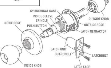
Optional thrubolts are provided and recommended for use on high frequency doors. Warranty voided if optional thrubolt are not installed.
