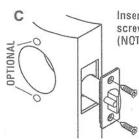
Insert latch and tighten screws.
