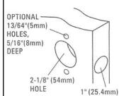
Drill 2-1/8" (54mm) hole through door face and two holes 13/64" (5mm), Drill 1" (25.4 mm) hole in center of door edge for latch. OPTIONAL:
